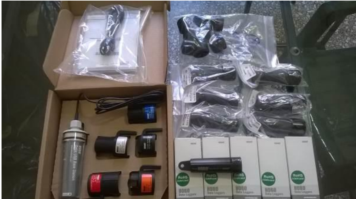
Figure 3: Onset's Waterproof Data Logger system which was installed at Zakynthos sampling sites for a long-term temperature monitoring.
